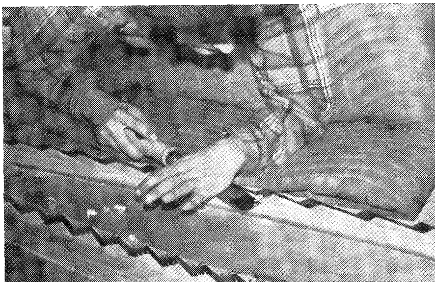
Position while notching bridge. Body weight is supported by left elbow on pad. Left elbow pivots and adds control to chisel while right arm and shoulder do the work. Safety precautions: Fingers and hands should be kept free from chisel blade and surface of bridge.
